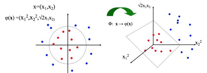
If data are mapped into higher a space of sufficiently high dimension, then they will in general be linearly separable; N data points are in general separable in a space of N-1 dimensions or more!!!
